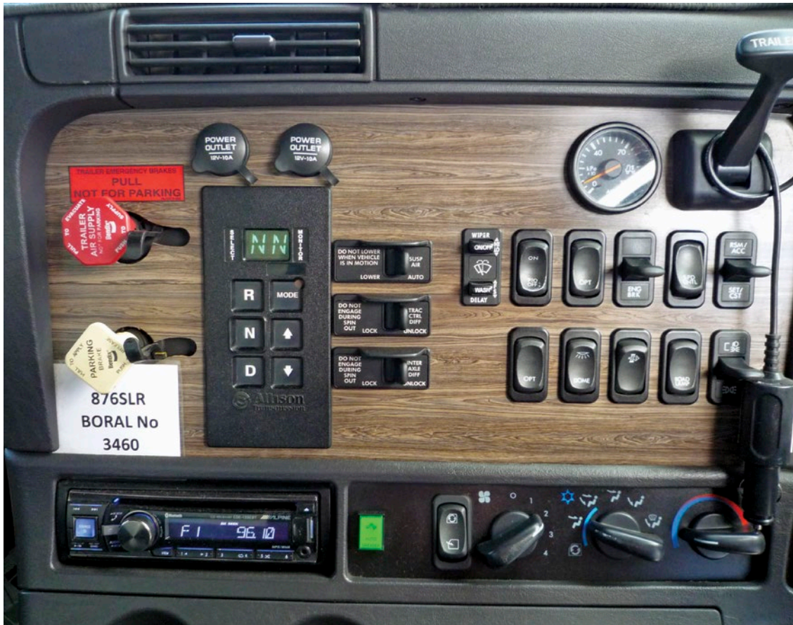
Left: The Allison Transmission touch pad style shift selector displays the requested gear and the current gear. The transmission oil level can also be checked by request via the MODE button.
